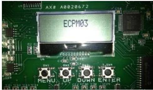
The ECPM03 board allows the user to configure a broad range of options associated with the functionality of the system through the setup menus on its LCD as shown above. Below the ECPM03 LCD are 4 buttons for navigation: MENU, UP, DOWN, ENTER.
